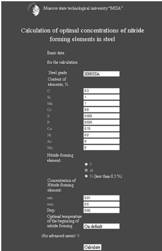
Fig. 2. Working window of the program of calculation of optimum concentration of nitride-forming elements in steel
