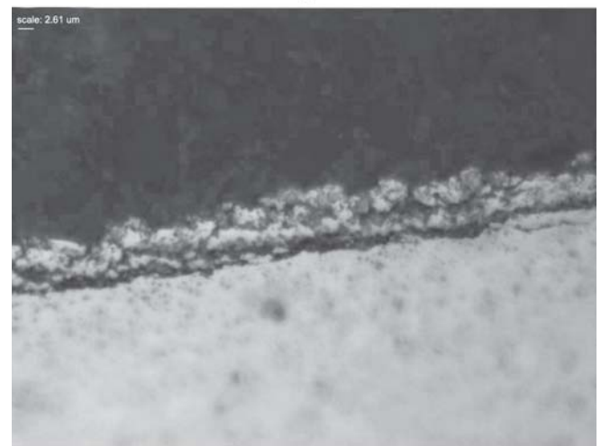
Fig. 3. Microstructure of Ta-coating (a - indicated arrow) electro-deposited on the surface of solid carbide insert and TaC-coating (b) formed by gas carburizing, x1000
