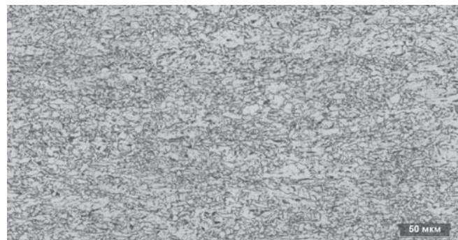
Fig. 8. Fracture surface of a sample after DWTT (a) and bainite microstructure corresponding with it (b). The magnification bar is 50 microns long
