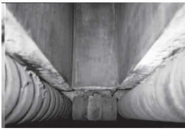
Fig. 1. R-7 Mold after removal from the CCM on stand
