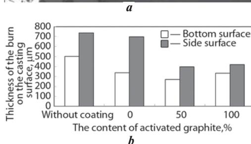
Fig. 3. Burning-on (a) and burning-on thickness on casting surface (b)
