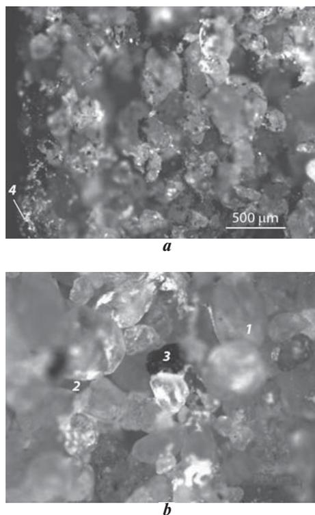
**Fig. 4. Schematic image of core section (a) and microstructure of samples painted by self-drying coating, containing 50% of natural graphite and 50% of mechanically activated graphite (a — edge; b — 0.5 mm from edge):**
