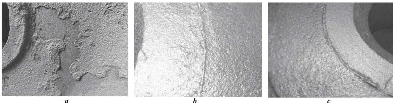
Fig. 2. Surface of the castings “Centrifugal soil pump. Internal pump shell”, fabricated without coating (a) and with coatings, containing 50% of graphite GLS-2 and 50% of graphite GLS-2A (b) and 100% of graphite GLS-2A (c)
