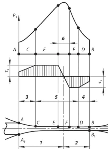
**Fig. 2. Distribution of contact normal and tangential stresses along the bite curve at  $l/h_{av} > 5$ :**
