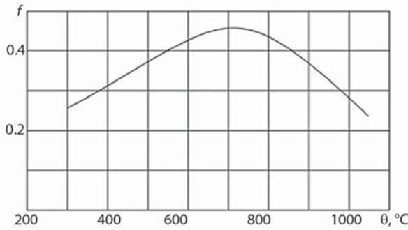
**Fig. 1. Relationship between friction coefficient and temperature [3]**
