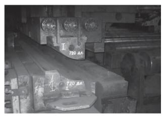
Fig. 1. The flanging press for steel sheet and its punch and matrix
