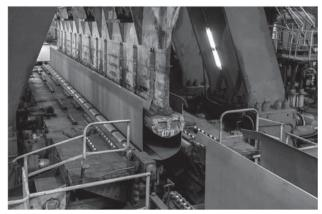
Fig. 2. The pre-shaping press TEWA 1020 for bending the central region of steel sheet
