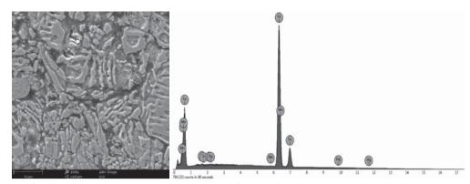
Fig. 2. Scanning microscope photograph and identification of elements present within the whole visible region covered by the photograph
