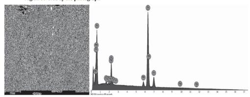
Fig. 3. Scanning microscope photograph and identification of elements present. The analysis was carried out in the spot marked with a "+"
