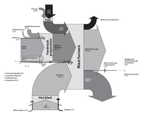
Fig. 1. Mass balance of blast furnace process. Stream values are referenced to 100 t of produced pig iron
