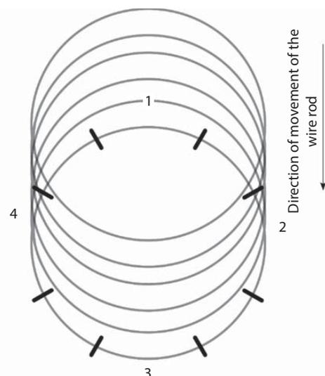
Fig. 1. Scheme of sample cutting
