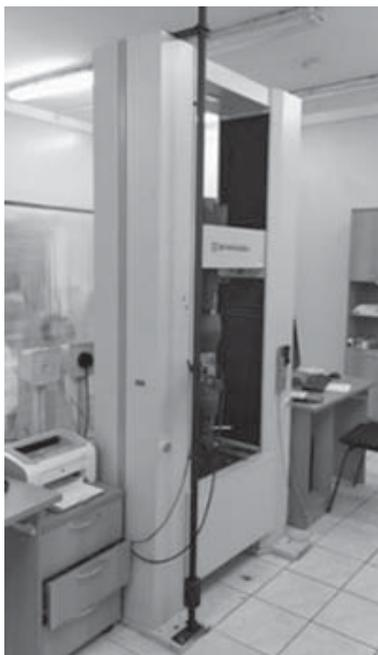
Fig. 2. Shimadzu AG-300KN-1 Universal Tensile Testing Machine
