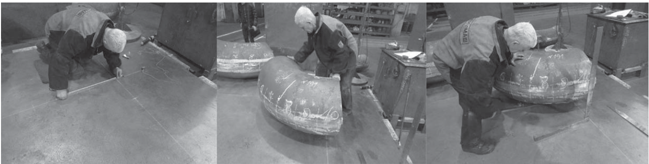
Fig. 1. The process of “lofting” technological operation during marking of a bend billet
