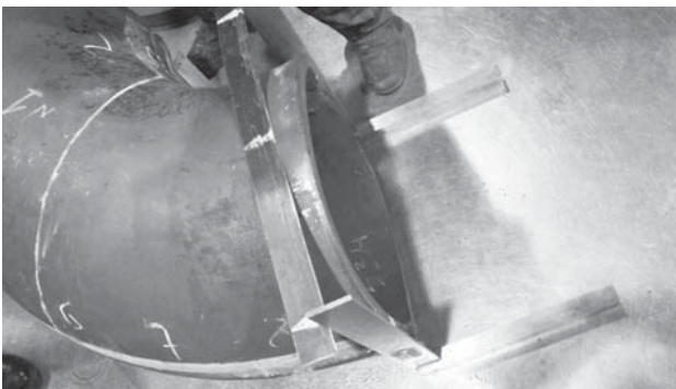
Fig. 2. Transfer of marking from a loft to a bend billet generatrix
