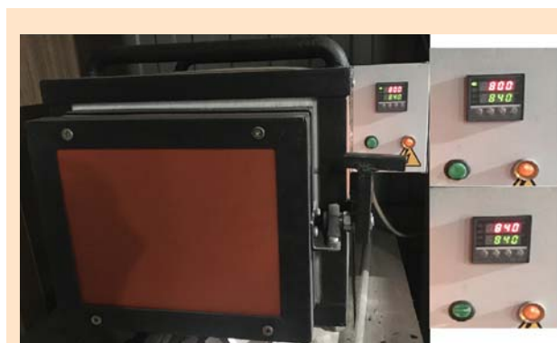
Fig. 6. Muffle furnace and its operating modes for the first kind of TC cycle
