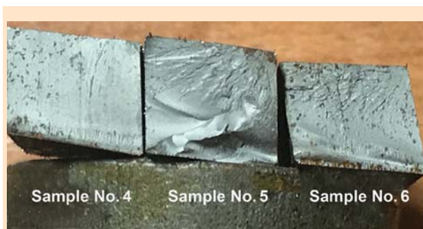
Fig. 8. Fracture surfaces of ShKh-15 steel samples No. 4–6
