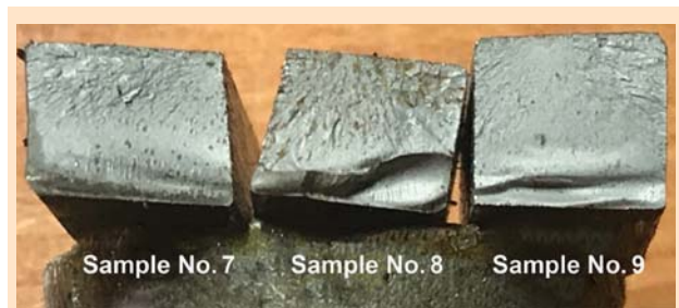
Fig. 9. Fracture surfaces of ShKh-15 steel samples No. 7–9
