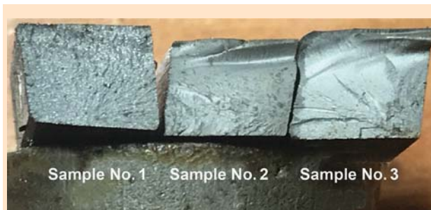
Fig. 7. Fracture surfaces of ShKh-15 steel samples No. 1–3
