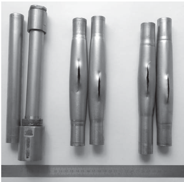
Fig. 3. The samples with the clamping grapples before the test ( a ); coupled samples, where the left one is tested by the instantaneous load, and the right with 5 min time-exposure ( b, c )
