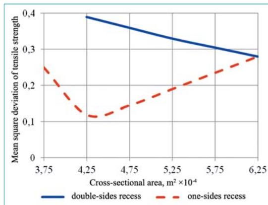
Fig. 9. Dependence of the standard deviation of the tensile strength of dry samples of the core mixture
