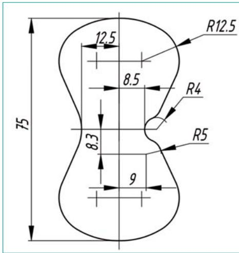
Fig. 6. Dimensions of sample with eccentric loading
