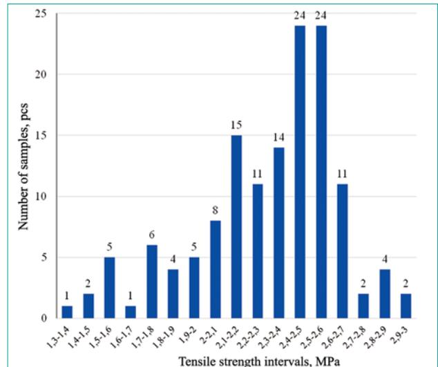
Fig. 3. Distribution of the number of samples by tensile strength intervals
