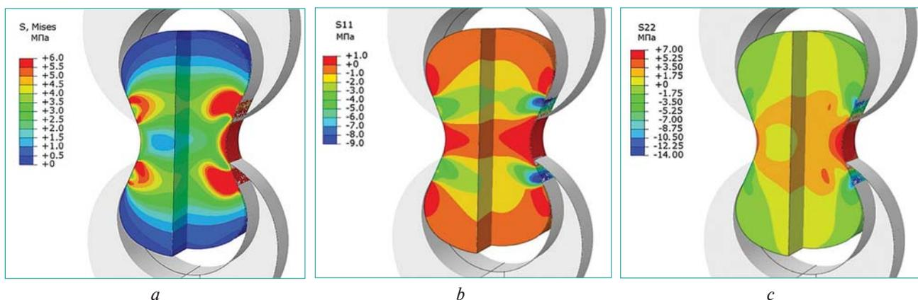
Fig. 5. Visualization of the formed stresses in the sample from the core mixture along the end surface and section views along the planes of symmetry: *a* – equivalent by Mises; *b* – horizontal component; *c* – vertical component
