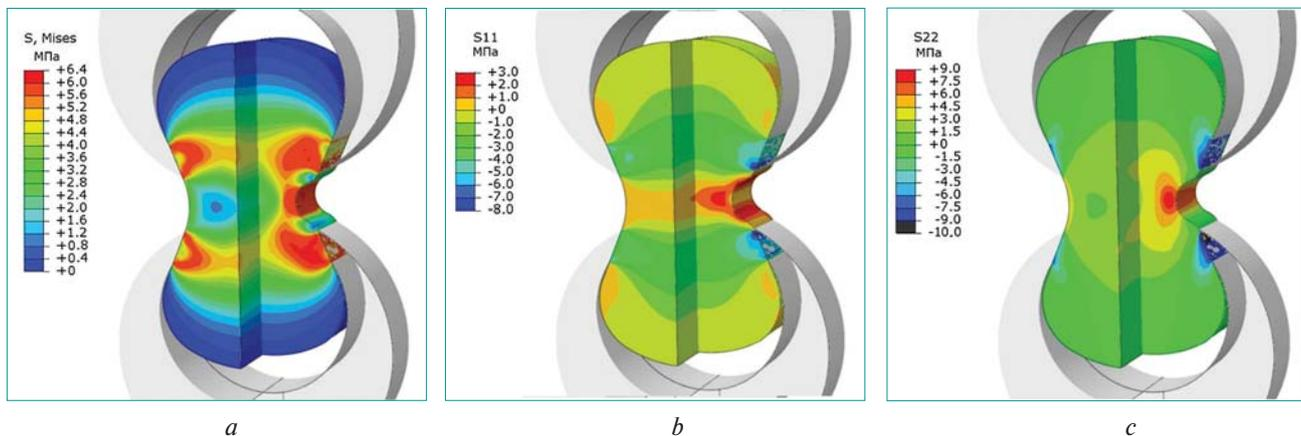
Fig. 8. Visualization of the formed stresses in the modified sample from the core mixture along the end surface and section views along the planes of symmetry:  $a$  – equivalent by Mises;  $b$  – horizontal component;  $c$  – vertical component
