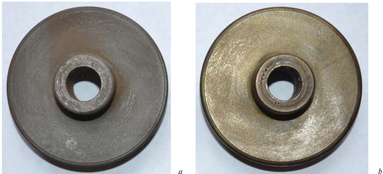
Fig. 3. The samples after testing for total hydrogen sulfide corrosion: a – without coating; b – with Ni–Cu coating
