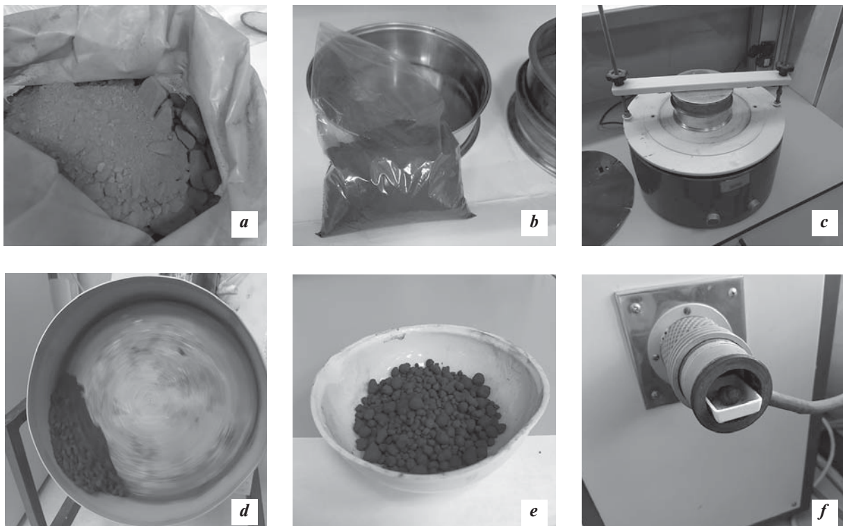
Fig. 3. The scheme of pellets obtaining from ferruginous quartzites in laboratorial conditions:
