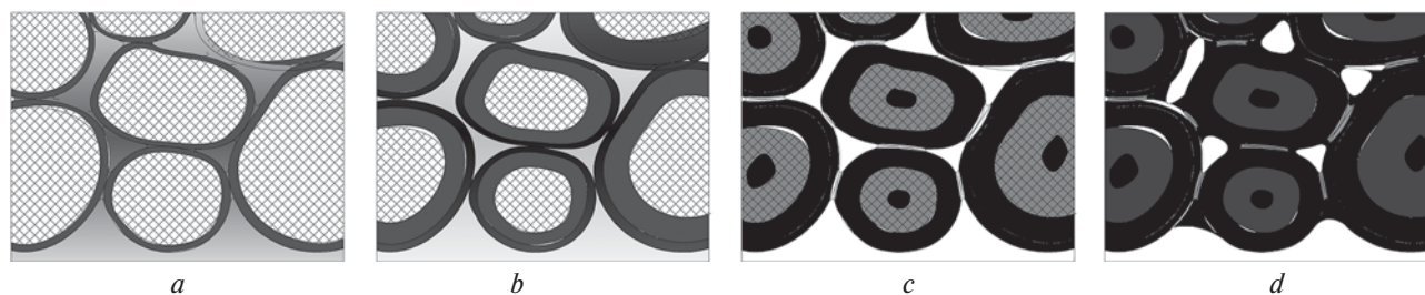
Fig. 2. The scheme of presentations of different bond types between a pellet grains:
