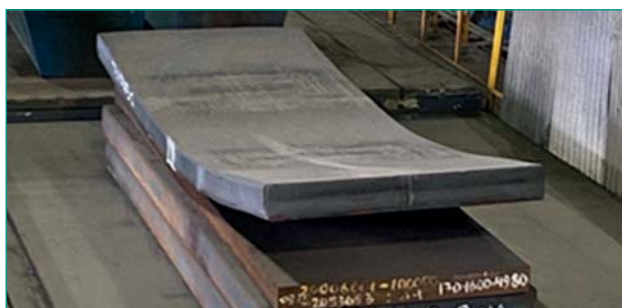
Fig. 1. Example of a deformed workpiece of alloyed steel grade 10KhGSN2MBF
