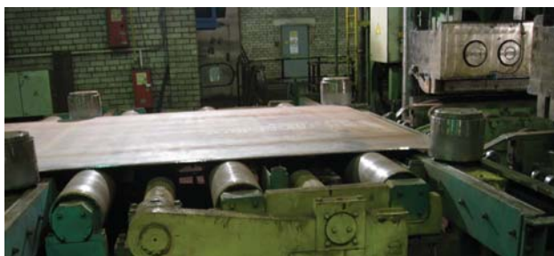
Fig. 1. Mechanism of feeding a steel sheet into edge-bending press
