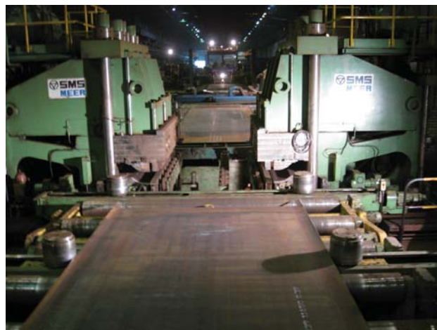
Fig. 2. Edge-bending press for deformation of steel sheet
