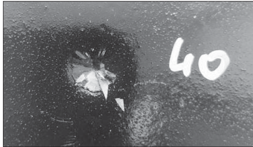
Fig. 4. Delamination of the coating P/E during strike of a flat die from the height 40 cm; after opening the polymer film, it is seen that the detachment occurred between the metal surface and polyurethane
