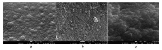
Fig. 4. The microstructure of the obtained protective coating of composition  $(Ti_{70.63}Al_{10.51}V_{6.85}Nb_{1.88}B_{16.14})_xO_y$  (example 3): a — before thermal annealing; b — after thermal annealing; c — after thermal annealing at high magnification
