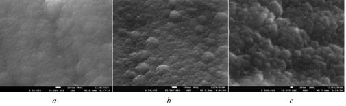
Fig. 3. Microstructure of the obtained protective coating of composition  $(Ti_{76.10}Al_{8.89}V_{5.99}Nb_{0.94}B_{8.07})_xO_y$  (example 1): a — before thermal annealing; b — after thermal annealing; c — after thermal annealing at high magnification
