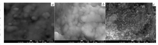
**Fig. 1. Microstructure of the obtained coatings:** a- nichrome Kh15N60; b- Ti6Al4VW alloy; c- thermally oxidized aluminum (Al $_2$ O $_3$ )
