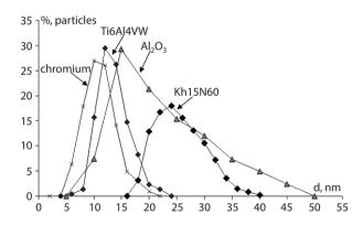
Fig. 2. Size distribution of nanoparticles in derived coatings
