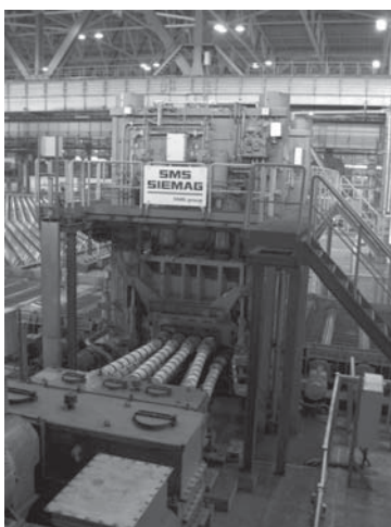
Fig. 1. The multi-roller straightening machine by SMS Siemag
