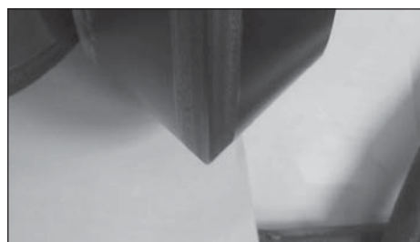
Fig. 4. Experimental dividing roller after rolling of 1,000 tons of rebars No. 12 in 370 mill
