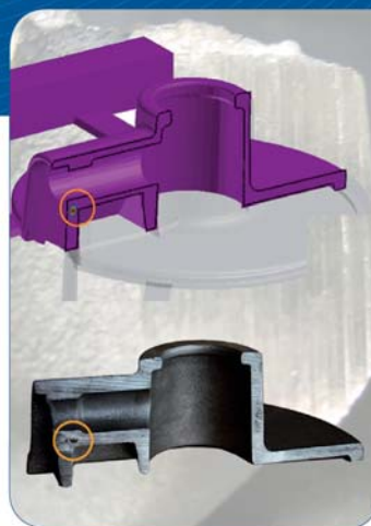
Predicted Shrinkage Porosity
