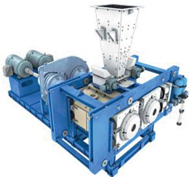
Fig. 1. HPGR: general view and structural components
