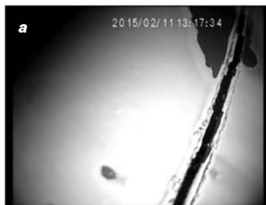
Fig. 2. (a) 7 mm wide crack in (b) the horizontal hole no. PN (Ø 59 mm, H = 750 m) 5.2 m downward of the hole mouth; distortion of the hole is observable
