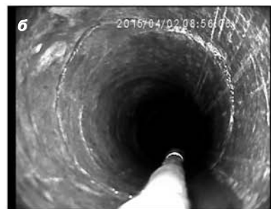
Fig. 2. (a) 7 mm wide crack in (b) the horizontal hole no. PN (Ø 59 mm, H = 750 m) 5.2 m downward of the hole mouth; distortion of the hole is observable
