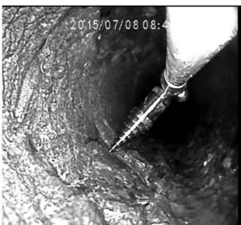
Fig. 3. Prod meant for measurement of width of a fracture and for estimation of fracture growth dynamics
