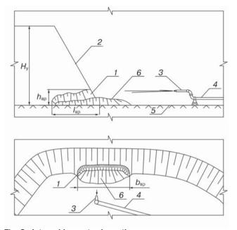
Fig. 2. Jet washing-out schematic: 1 - cut; 2 - face slope: 3 - jet; 4 - water line; 5 - bed rock; 6 - washed-out rock
