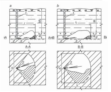
Fig. 1. Sector-like shape of a stope: a - short; b - long:
