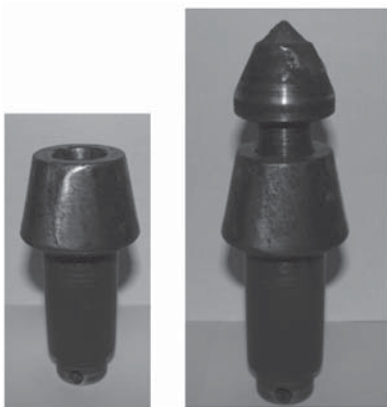
Fig. 5. Reconditioned pick: a — holder from rejects; b — installation of replaceable nose
