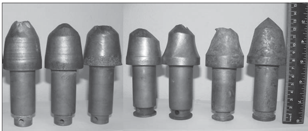
Fig. 1. Worn-out picks of coal cutting machines
