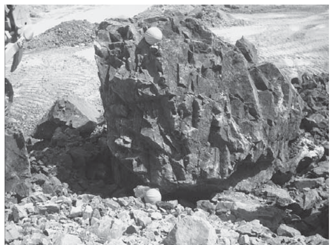
Fig. 3. Effects of uncertainty on oversize block formation and inefficient blasting results in Sungun Copper Mine (in the right photo the diameter of green plastic balls are 17 cm)
