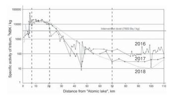
Fig. 4. Concentration of tritium (<sup>3</sup>H) in the Shagan River versus distance from the Atomic Lake
