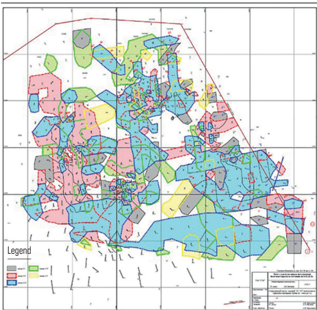
Fig. 2. Co-located contour map of ore deposits in the depth range from +340 m to 0 m
