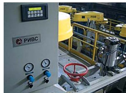
Fig. 2. Flotation machine RIF 16 equipped with the system ASSUP-RV
