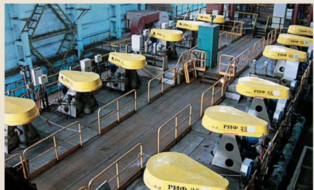
Section of flotation final treatment of the magnetite concentrates at Inguletsky GOK, Krivoy Rog, Ukraine
