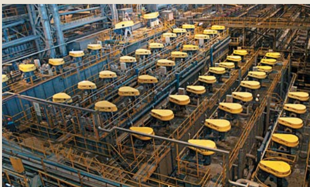
Second section of the collective cycle of the copper-molybdenum flotation. KOO "Enterprise "Erdenet", Mongolia
