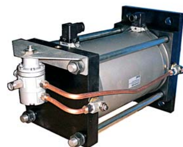
Fig. 10. Pneumatic drive of the bottom slide-valve with the system of braking
