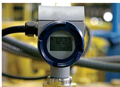
Fig. 9. Sensor of pressure with the digital indication of the current value
