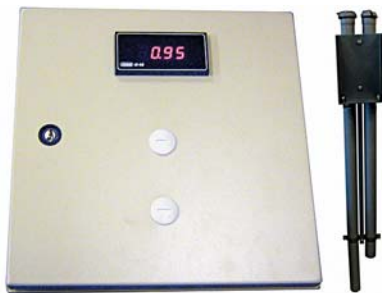
Fig. 11. Indicator of density (PIP-RIF). The box with converter and measuring counter
