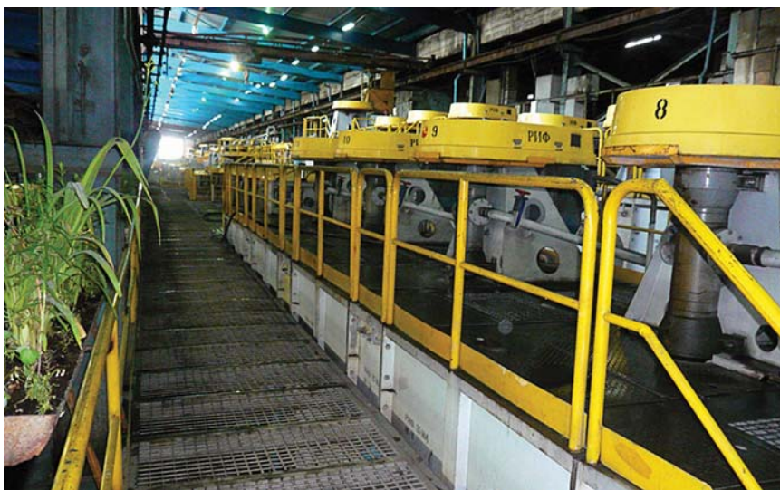
Fig. 2. Flotation section with flotation machines RIF
