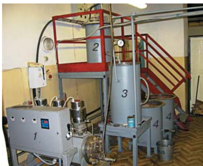
Fig. 3. Experimental-industrial unit for zinc removal from the copper concentrate
