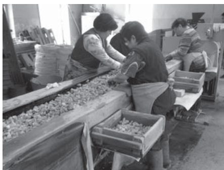
Fig. 2. Additional manual sorting of separation concentrate
