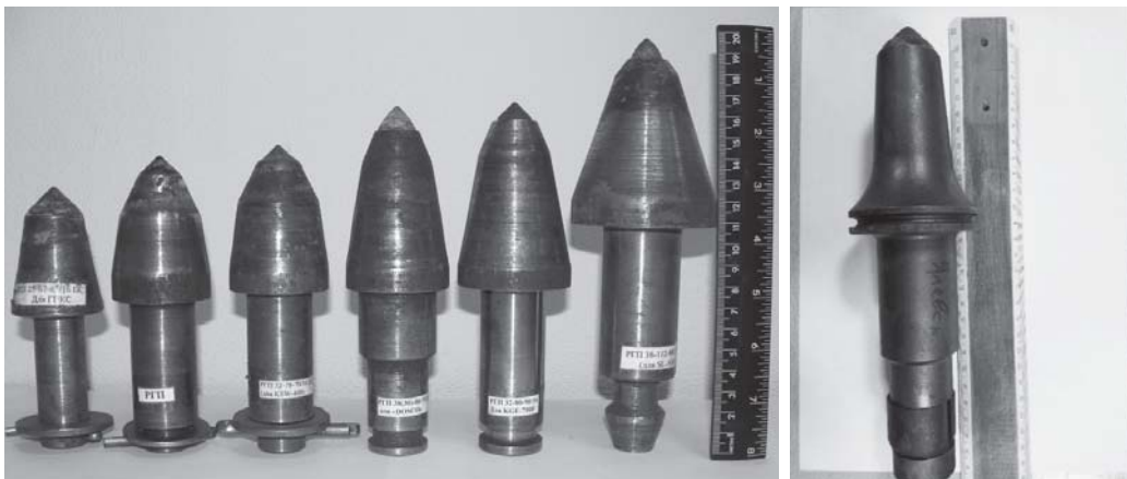
Fig. 1. Change in dimensions of picks for cutter-loaders.
