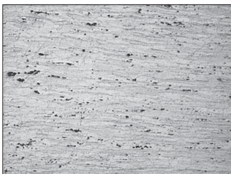
Fig. 2. The microstructure of the annealed AMg6 alloy (×100)
