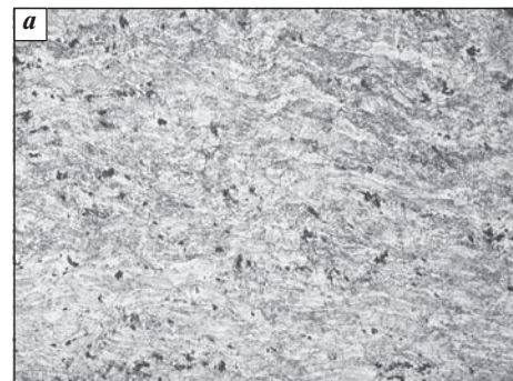
Fig. 9. The AMg6 alloy microhardness after shear-compression processing at a temperature of 200 °C
