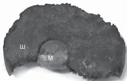
Fig. 2. The outward appearance of the product of red mud reducing roasting under optimal conditions M — metal, Ш — slag
