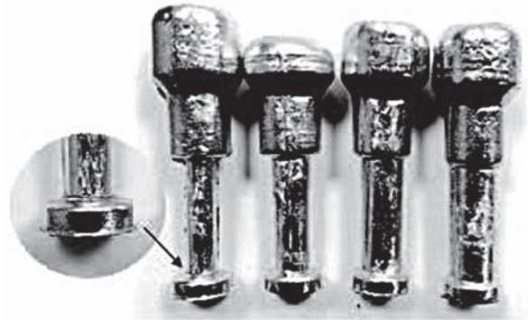
Fig. 3. Cast Al6Ca4La2Mn alloy samples 10 to 16 mm in diameter obtained using the pencil test
