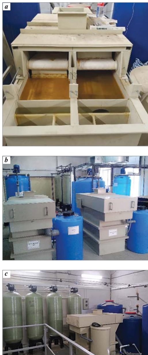
Fig. 2. The production pieces of equipment, output: a — 1 \text{m}^3/\text{h} ; b — 5 \text{m}^3/\text{h} ; c — 10 \text{m}^3/\text{h}
