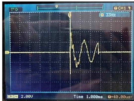
Fig. 8. Typical oscillograms of a discharge with different pulse durations on GIT TNM 1-2
