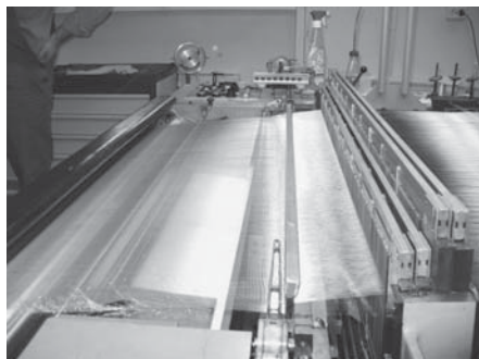
Fig. 6. The production process of woven gauze, Type 3
