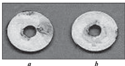
Fig. 2. An outward appearance of the samples without coating after the tests: a — non-magnetized sample; b — magnetized sample
