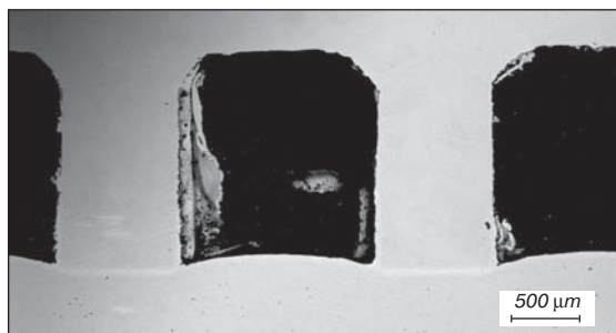
Fig. 9. Microstructure of mock-up samples obtained at 1150 °C for 30 minutes
