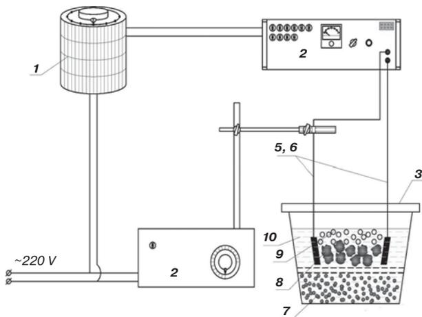
**Fig. 1.** Schematic diagram of electroerosion dispersion of T5K10 alloy waste:
