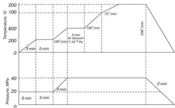
**Fig. 3.** Scheme of consolidation of powders by SPS method
