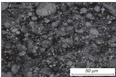
**Fig. 2.** Scanning electron microscopic image of electroerosive hard alloy powders
