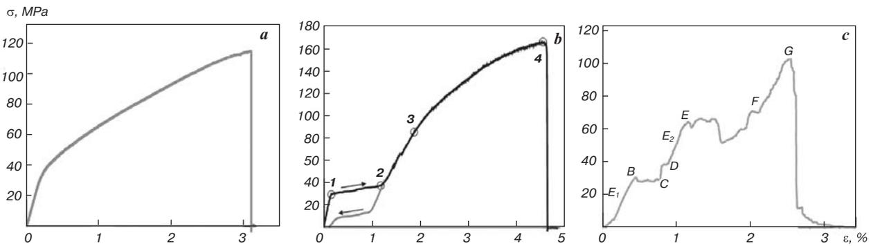
**Fig. 2.** Typical deformation diagrams, obtained by uniaxial stretching of porous plates of titanium nickelide: a – 20×12×6 mm; b – 20×12×3 mm; c – 20×12×0.5 mm
