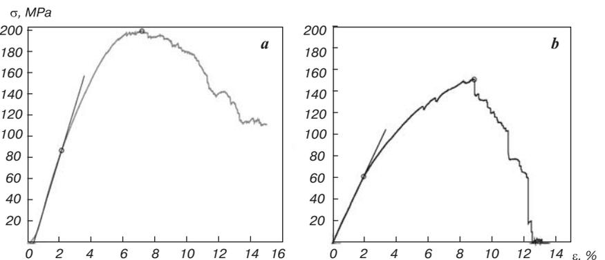
**Fig. 1.** Typical deformation diagrams obtained by uniaxial quasi-static compression of SHS-alloys of porous titanium nickelide: a – 12×6×6 mm; b – 6×3×3 mm
