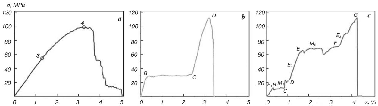
Fig. 4. Typical deformational diagrams obtained by three-point bending of porous plates from titanium nickelide: a – 30×10×5 mm; b – 30×10×3 mm; c – 30×10×0.5 mm
