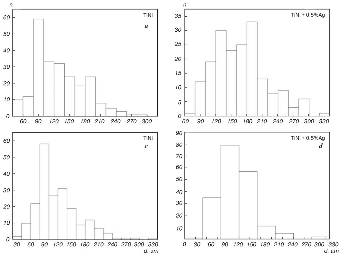
Fig. 4. Histograms of the size distribution of (a, b) – pores; (c, d) – interporous bridges in the samples of the TiNi porous SHS-alloy
