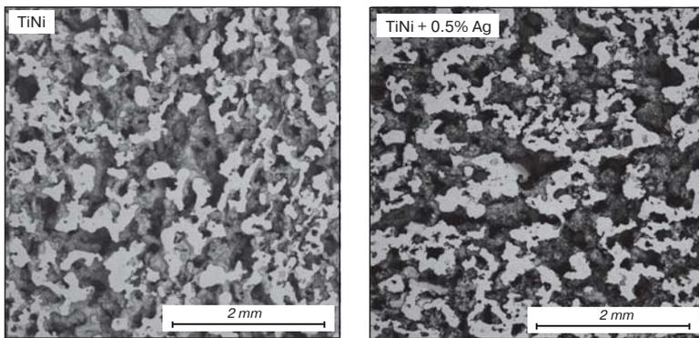
Fig. 3. Raster images of the sample surfaces of the TiNi porous SHS-alloy
