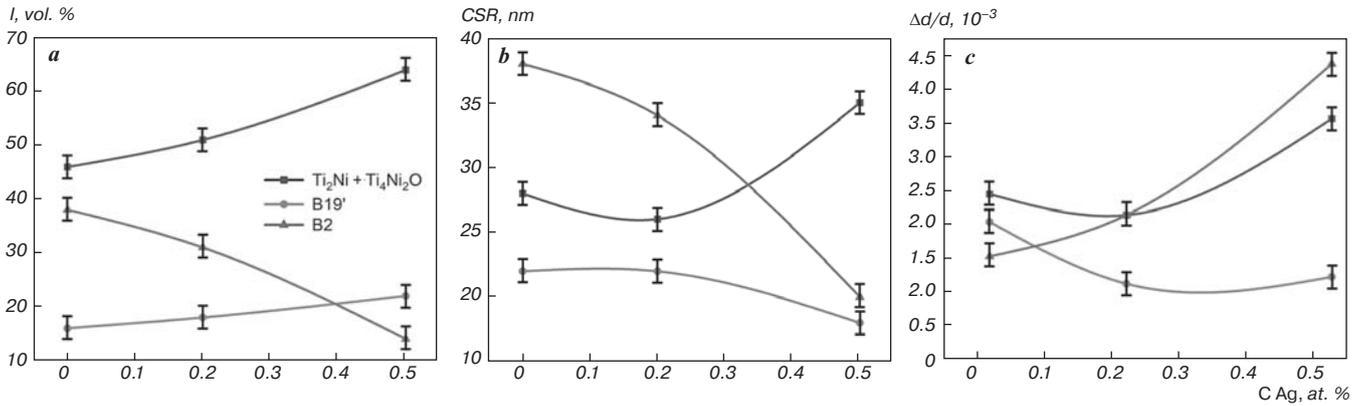
Fig. 2. Concentration dependence based on the results of the X-ray diffraction analysis of the samples of the TiNiAg porous SHS-alloy: a – volume fraction of phases; b – CSR values; c – micro-distortions
