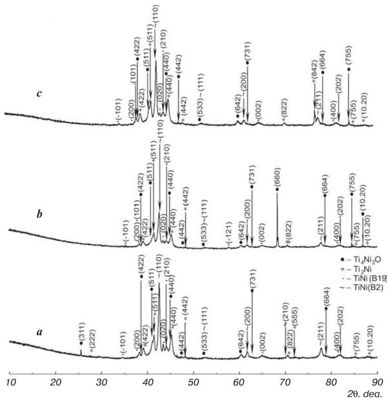
Fig. 1. X-ray diffractograms of TiNi porous SHS-alloy samples for: a - TiNi; b - TiNi + 0.2%Ag; c - TiNi + 0.5%Ag
