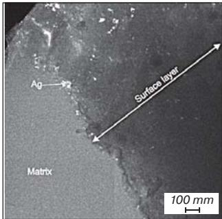
Fig. 9. Transmission electron microscopy and element mapping of the TiNi + 0.5%Ag porous SHS-alloy
