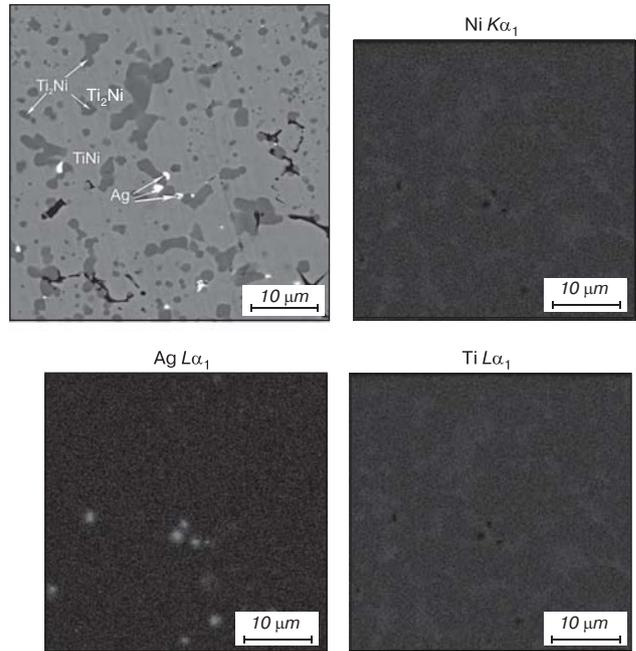
**Fig. 6.** Raster image of the microstructure and mapping by the chemical elements of the TiNi + 0.2%Ag porous SHS-alloy
