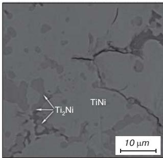
**Fig. 5.** Raster image of the microstructure and mapping by the chemical elements of the TiNi control porous SHS-alloy
