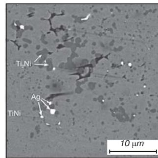
**Fig. 7.** Raster image of the microstructure and mapping by the chemical elements of the TiNi + 0.5%Ag porous SHS-alloy
