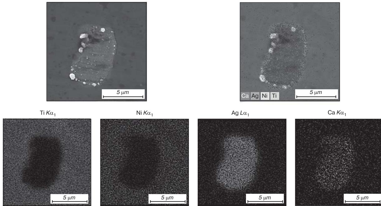
**Fig. 8.** Raster image of the microstructure and mapping by the chemical elements of the CaAg particle in the TiNi + 0.5%Ag porous SHS-alloy
