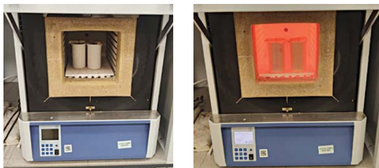
Fig. 1. LOIP muffle furnace with the loaded samples (in ceramic crucibles) in course of the oxidative test
