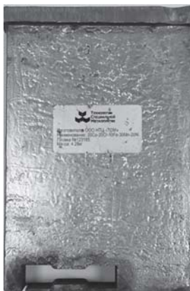
Fig. 1. \text{Co}_{20}\text{Cr}_{20}\text{Fe}_{10}\text{Mn}_{30}\text{Ni}_{20} alloy ingot and specimen size for uniaxial tensile testing
