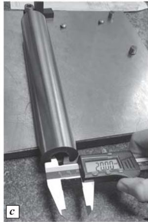
Fig. 2. General views of the upper edge of a TiNi SMA shell (a), TiNi SMA shell with an outer diameter of 40.0 mm and a tubes schedule of 10.0 mm (b), TiNi SMA rod with a diameter of 14.5 mm (c) after cutting on a SCT32-ST electrical discharge machine (photo by authors)
