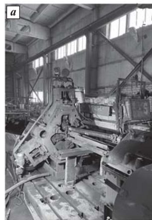
Fig. 3. General views of the screw rolling mill SVP 70 (a), the TiNi SMA shell during plugging on the SVP 70 screw rolling mill (b) and after the first pass (c) (photo by authors)
